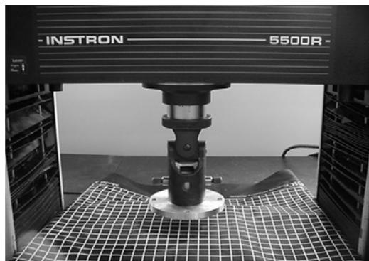
Figure 2 – Set up of a pressure pad in the Instron 5500R.
